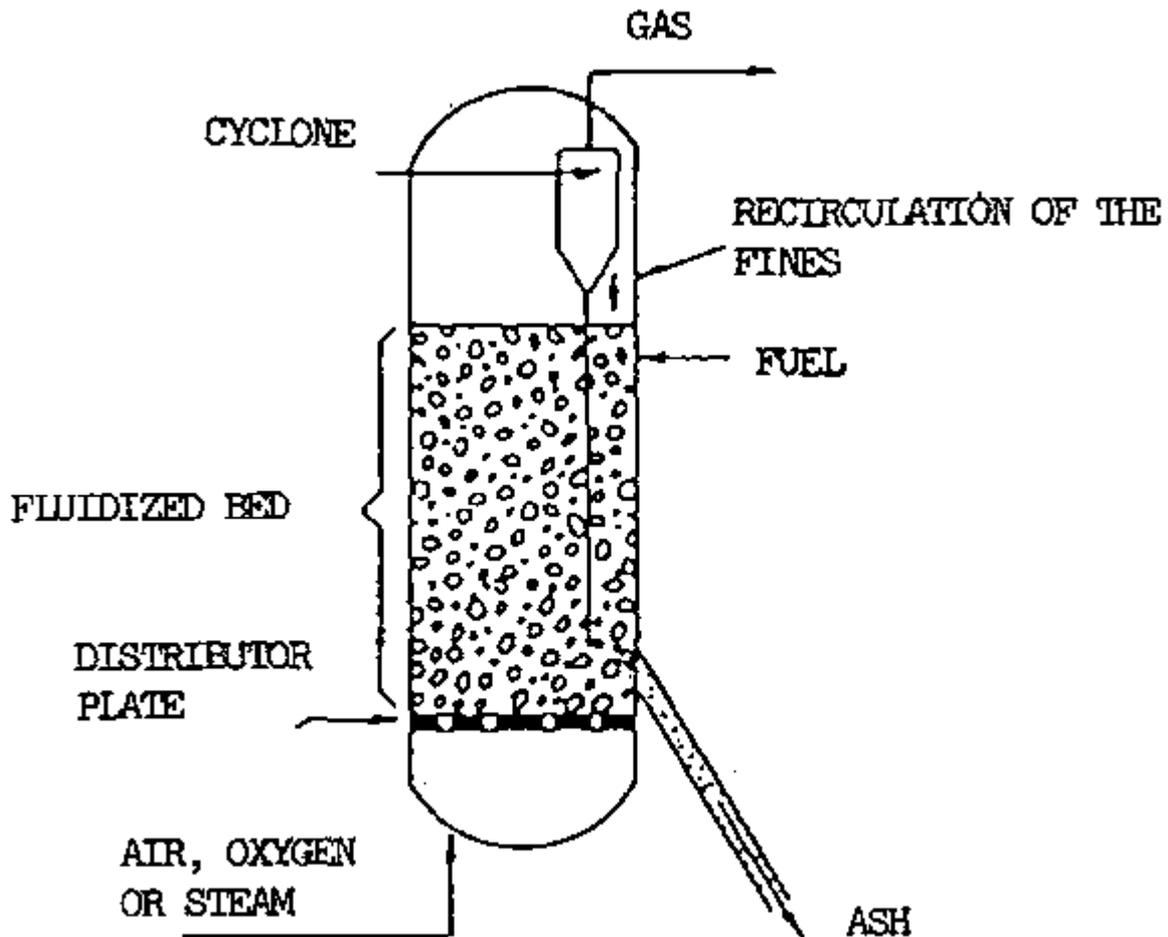
The major advantages of fluidized bed gasifiers, as reported by Van der Aarsen (44) and others, stem from their feedstock flexibility resulting from easy control of temperature, which can be kept below the melting or fusion point of the ash (rice husks), and their ability to deal with fluffy and fine grained materials (sawdust etc.) without the need of pre-processing. Problems with feeding, instability of the bed and fly-ash sintering in the gas channels can occur with some biomass fuels.
