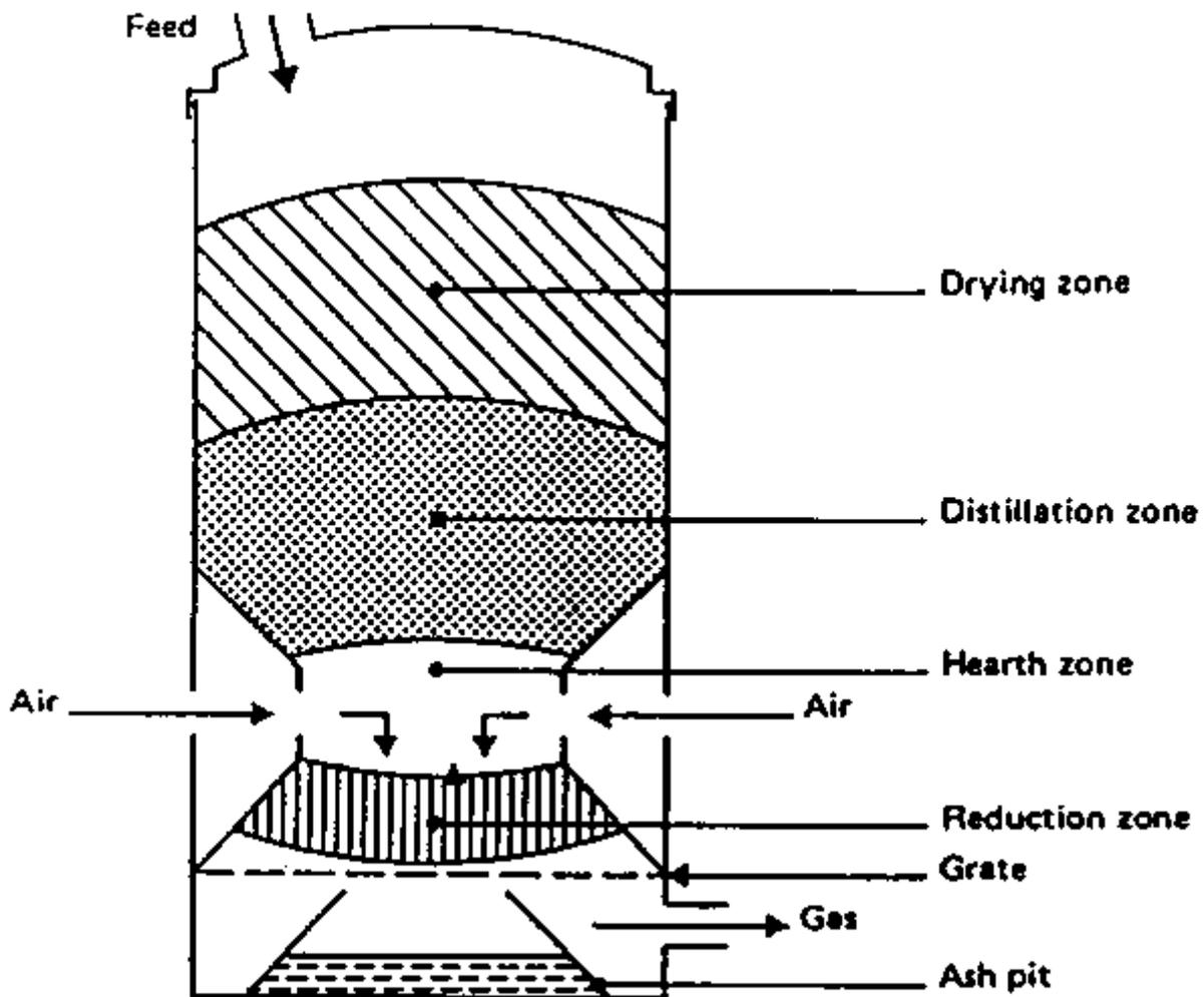
On their way down the acid and tarry distillation products from the fuel must pass through a glowing bed of charcoal and therefore are converted into permanent gases hydrogen, carbon dioxide, carbon monoxide and methane.
