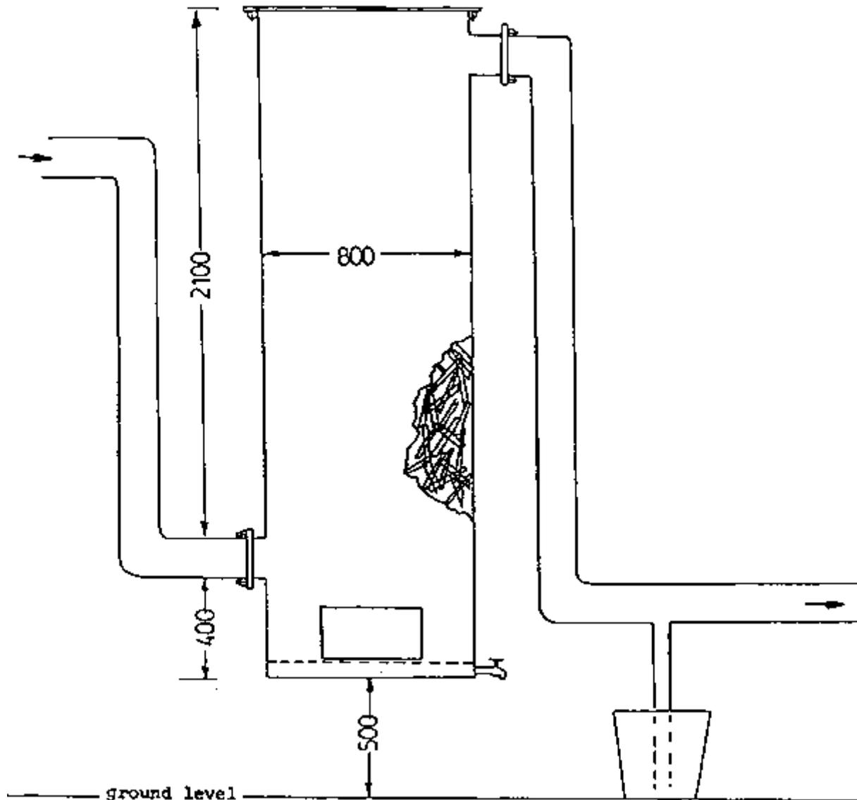
The construction of the filter is simple and practical and ensures a long working life, the filter material being changed every two years of operation.
