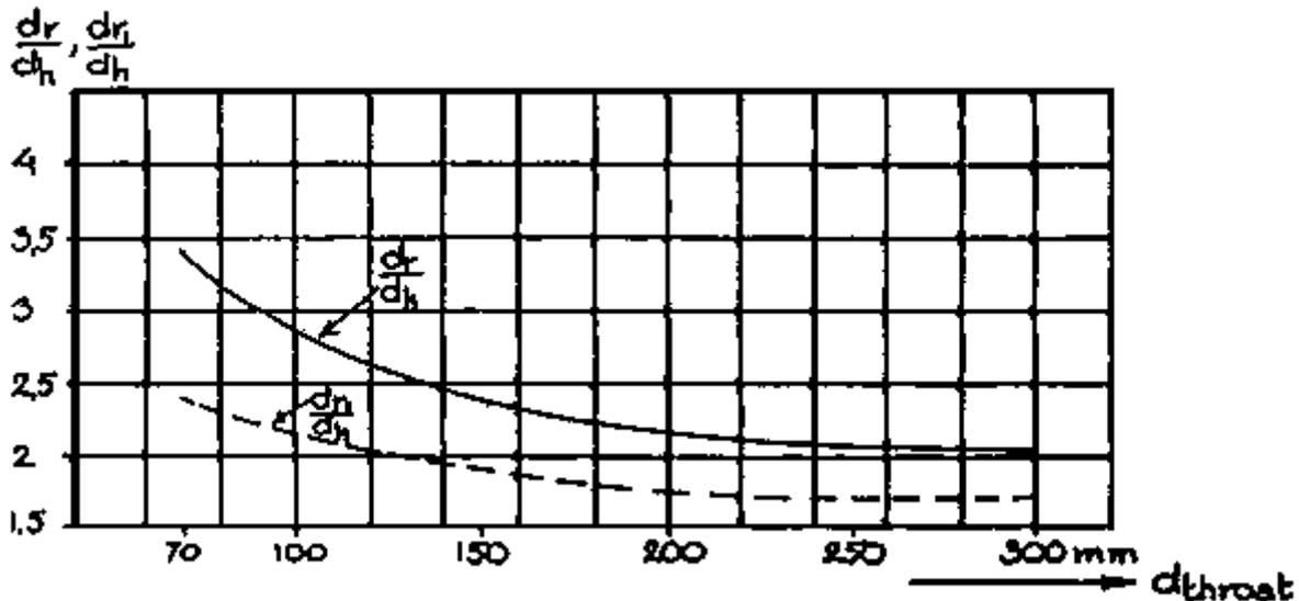
Venselaar (46) compares the design characteristics of a number of gasifiers that were commercially available during the Second World War. A distinction is made between "no throat" "single throat" and "double throat" (Imbert type) designs (see Figure 2.15). He comes to the conclusion that the three types differ mainly in maximum allowable hearth load, giving values of  $B_{max}$  of 0.03, 0.11 and 0.4, respectively for "no throat", "single throat" and "double throat" gasifiers.
